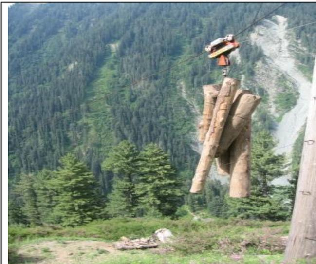
Figure 3: Timber extraction through cable cranes in Moist Temperate Forests in Pakistan
