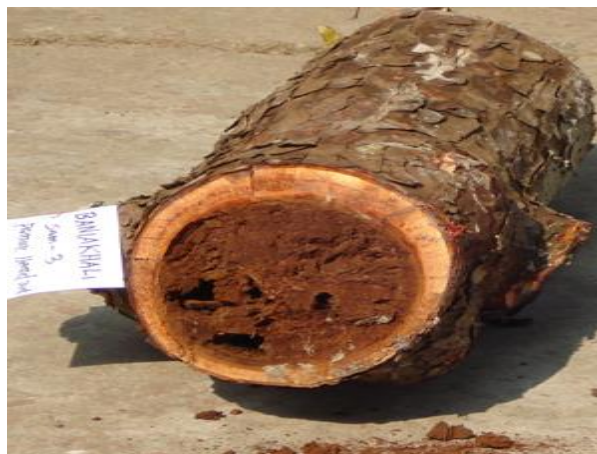
Fig.11: Heart rot damaged Passur log
